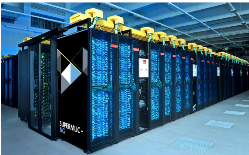
A Fahrenheit adsorption chiller converts the heat generated by the processors of the SuperMUC-NG supercomputer into cooling energy so that the computer uses it to cool itself.
